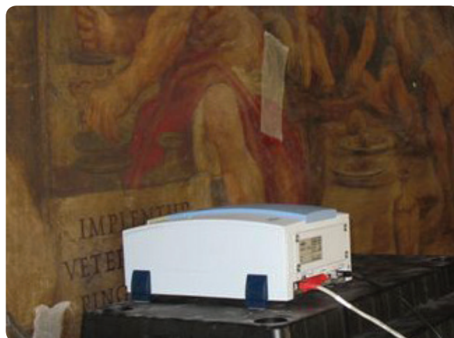
ALPHA II™ FT-IR analyzer investigating a mural painting by Francesco Albani in Bologna, Italy
