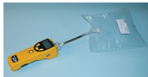
Gas sampling bag used for PID calibration.
