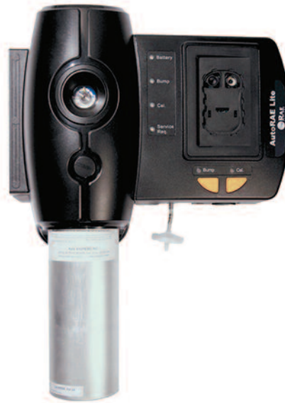
Bump testing ToxiRAE 3 with AutoRAE Lite for ToxiRAE 3 Bump Test and Calibration Station
