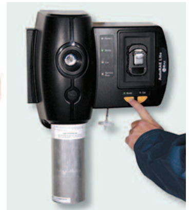
Bump testing ToxiRAE 3 with AutoRAE Lite for ToxiRAE 3 Bump Test and Calibration Station
