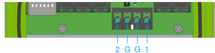
Figure 15: Tank/Well Float Switch
