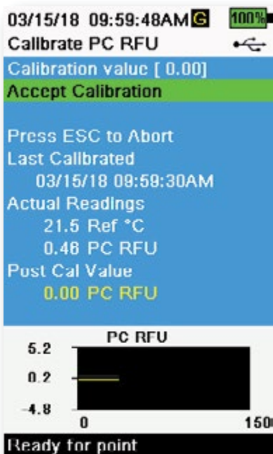
Figure 58 Calibrate PC RFU
