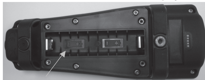
Figure 1. ProODO with battery cover removed. Notice battery symbols indicating polarities.
