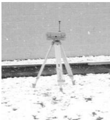
Figure B-13: Enclosure Mounted on a Tripod.
