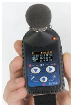
Figure 2-1 SV 104 instrument with the microphone and windshield
