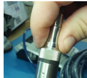
Properly completed—black ring uncompressed
