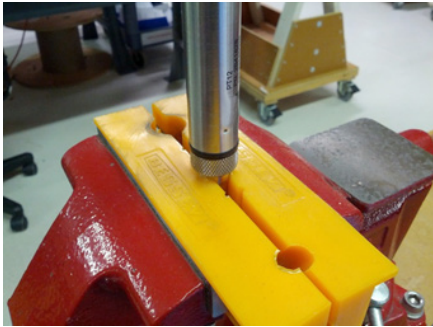
Cabled Sensor—gripping on swage
