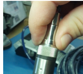
Properly completed—black ring uncompressed
