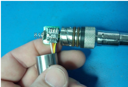
Connector connected properly
