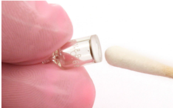
Figure 12: Polishing the Electrode Lamp Window
