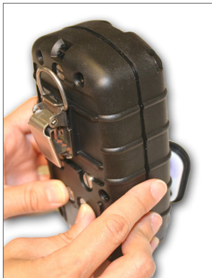
Figure 14. Pushing screws to remove sensor cover.
