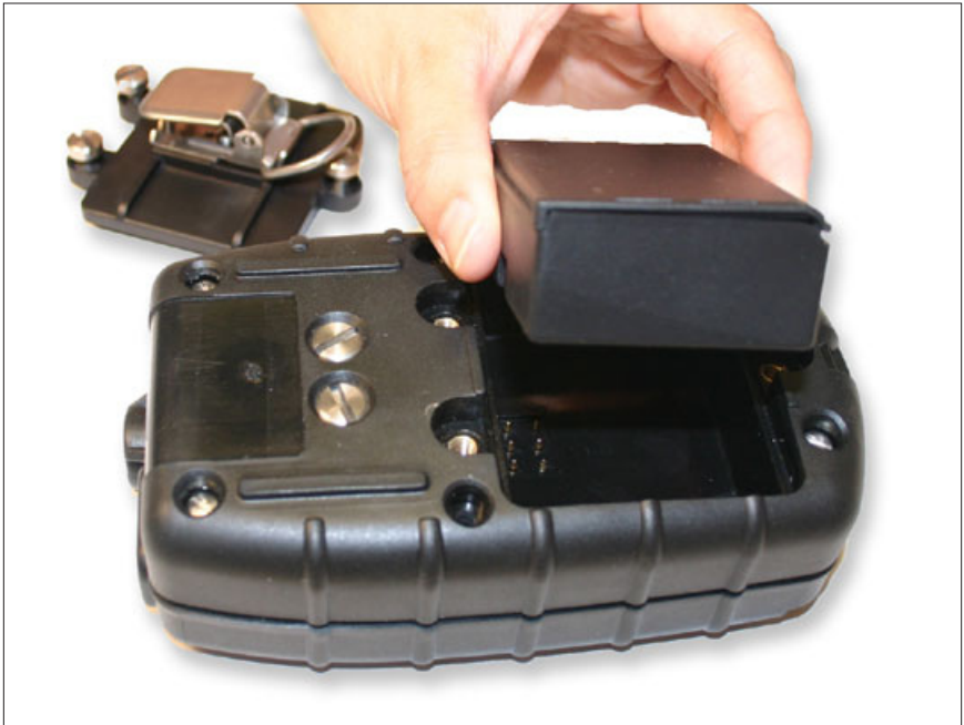
Figure 10. Removing the Li-Ion Battery Pack.
