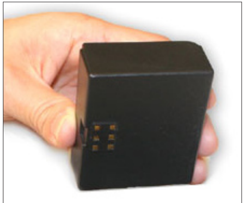
Figure 7. Contacts on the battery pack.
