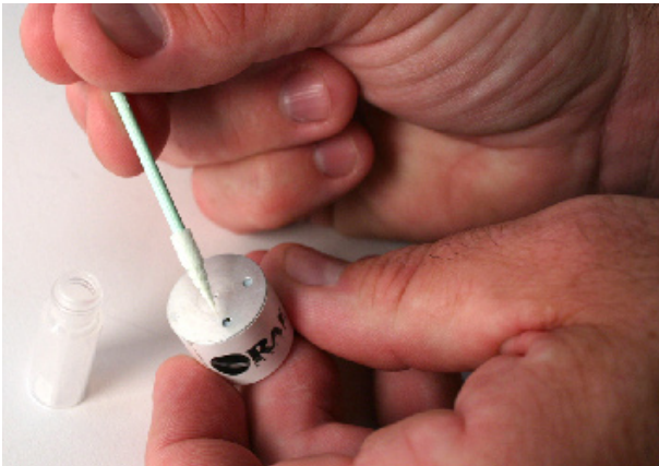
Figures 19. Cleaning the PID.
