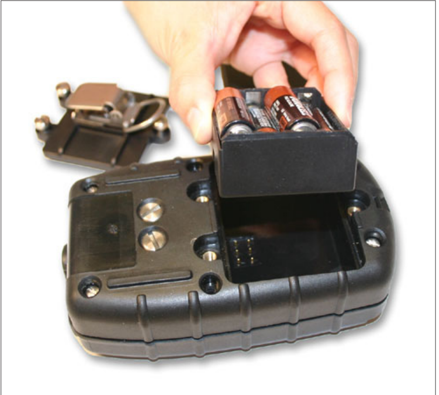
Figure 11. Installing the Alkaline Battery Pack.
