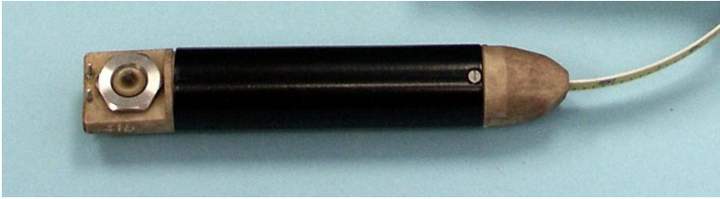
Figure 1-5: Large Diameter Chemical Interface Probe
