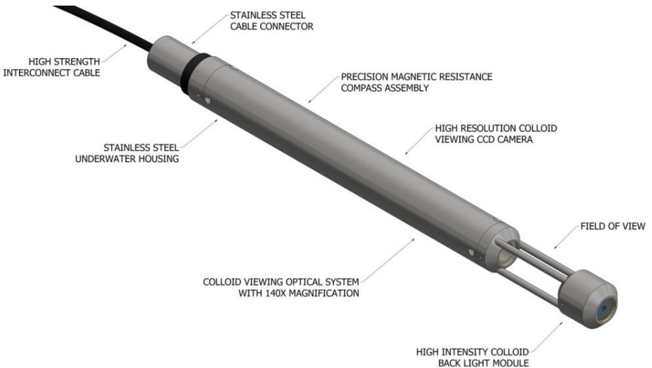
Figure 1-1: Colloidal Borescope Probe Features
