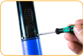
Tighten screw at base of each sensor with Allen wrench.
