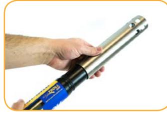
After calibration, flip the restrictor 180 degrees for deployment.
