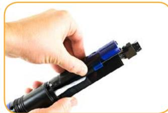
Insert RDO sensor in instrument sensor port.
