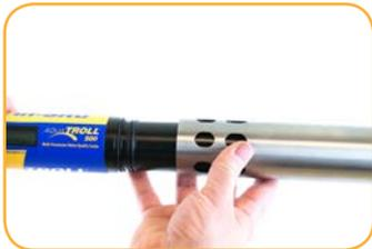
Remove the restrictor from the instrument.
