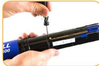
Place Allen wrench in the small hole at the bottom of the sensor.
