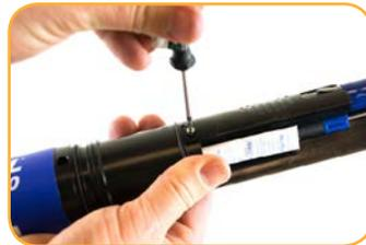
Use included Allen wrench to loosen set screw on RDO sensor.
