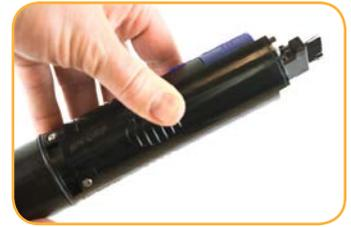
Insert pH/ORP sensor in empty sensor port.
