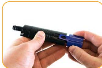
Install the RDO cap on the sensor.
