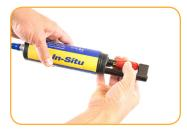
Remove the dust cap from the RDO sensor.
