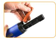
Remove the orange plug from the pH/ORP sensor port.
