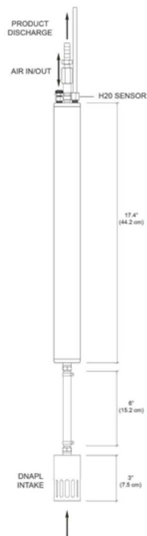
Figure 1-3: DNAPL recovery configuration for Stainless Steel Pump
