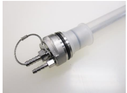
Figure 4-14b: Compression ring secured
