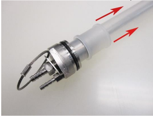
Figure 4-3: Removal of upper Compression Ring
