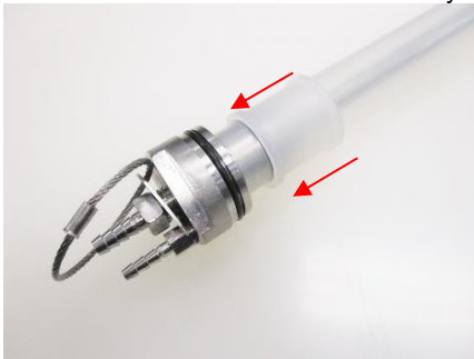
Figure 4-14a: Compression Ring on Bladder
