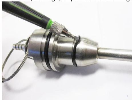
Figure 4-5: Removal of O-rings
