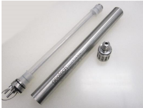
Figure 4-1: Removal of the bottom intake and outer housing
