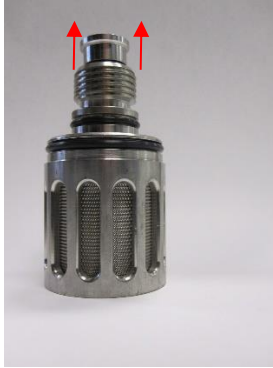
Figure 4-7b: Removing Check Ball Retainer
