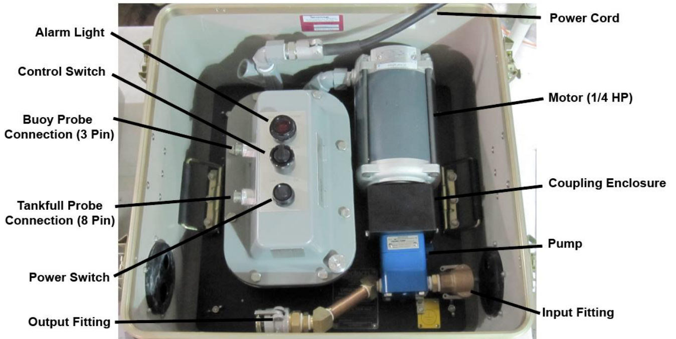
Figure 1-4: New LDFS Pump Control Module Assembly
