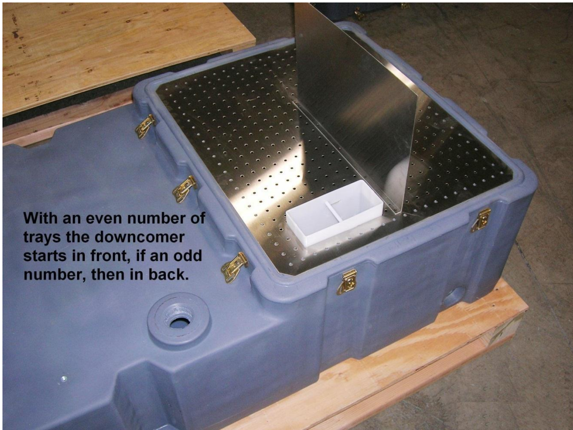
Figure 4-3: First Bubble Plate on Sump
