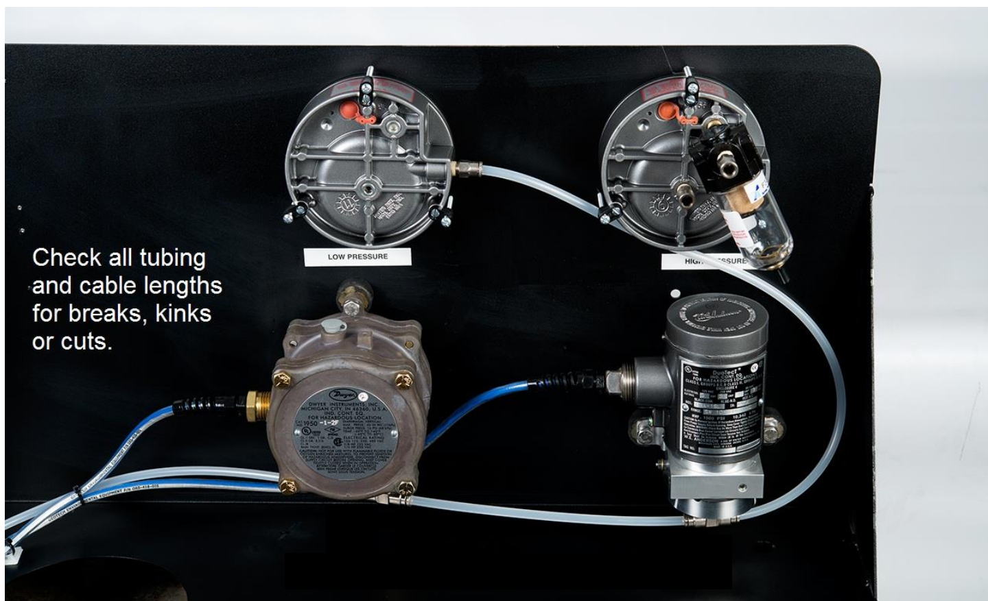
Figure 4-4: Static Sensor Tubing between gauges and switches (CFM gauge tubing not shown)
