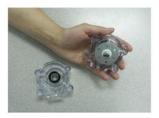
2. Place the tubing around the rollers.
