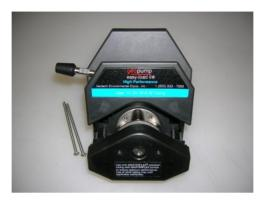
3. Set the lever to the right to close the pump housing onto the tubing.
