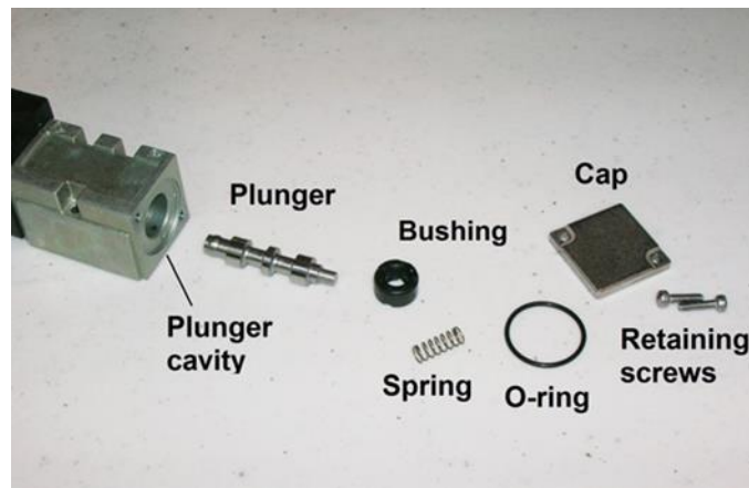
Figure 5-3: Solenoid Parts
