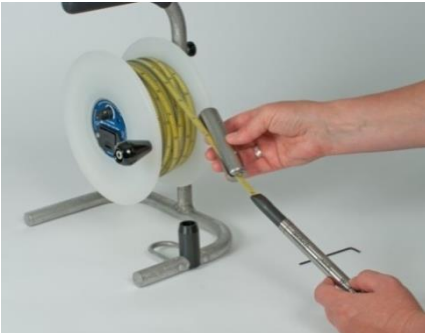
Figure 2-2: Fitting (Optional) Tape Weight
