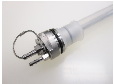
Figure 4-14b: Compression ring secured
