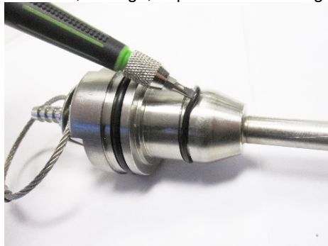
Figure 4-5: Removal of O-rings
