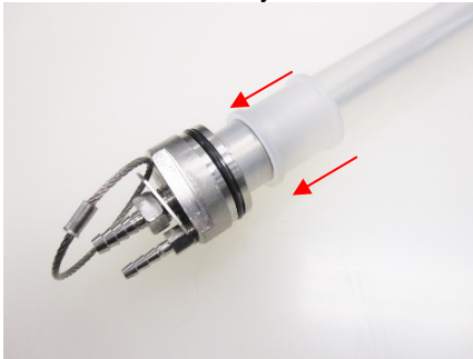
Figure 4-14a: Compression Ring on Bladder
