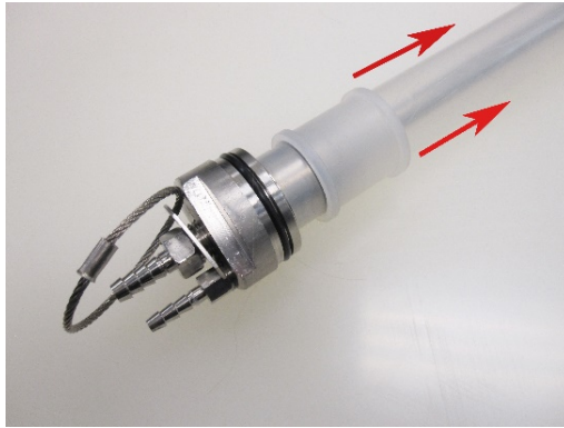
Figure 4-3: Removal of upper Compression Ring
