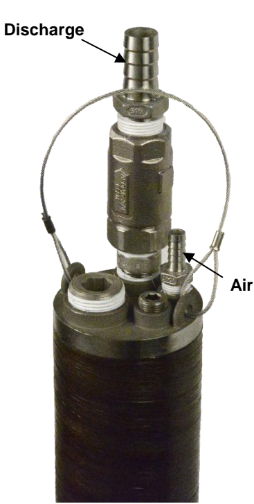
Figure 2-1: 3.5 Reclaimer Bottom Fill
