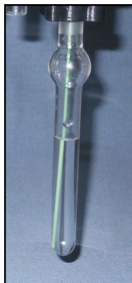
Figure 8.1-4: Look for Bubbles in the sparge bottle.
