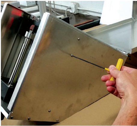
Remove cover screws with Allen wrench
